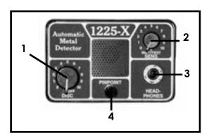
Figure 3. Control Panel. Two knobs and a button do it all.
